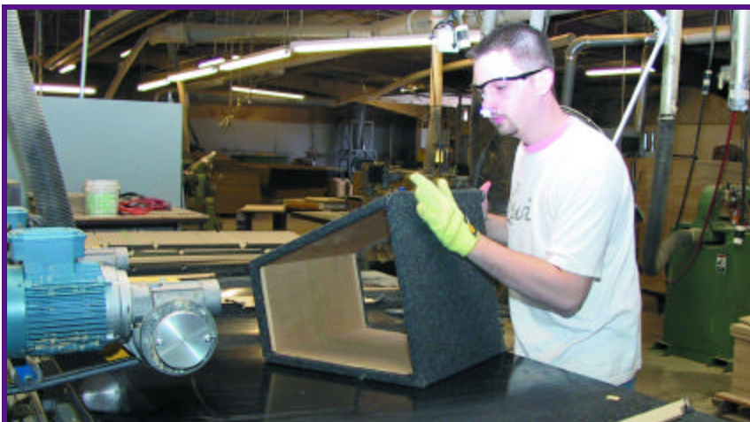
At the finish, an operator takes the piece, trims off edges, makes sure the piece is cut right and stacks it on a conveyor to go to the CNC router for further machining.
