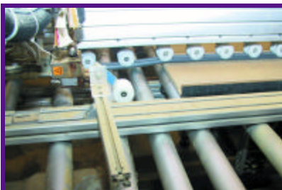
A close-up of the rollers and v-grooving in action. What starts out as a flat panel ends up with curved edges and dados.
