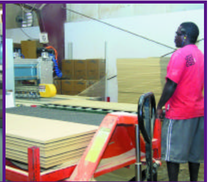
Panels are fed into the v-grooving lineal line, carpet side down. The v-groover has 11 cutterheads on it, seven fences and a roller system on each side.
