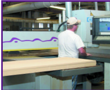
After panels are laminated with carpet on one side the panels are cut to size with the Holzma beam saw. Cut panels are very close to the finished size of the speaker.
